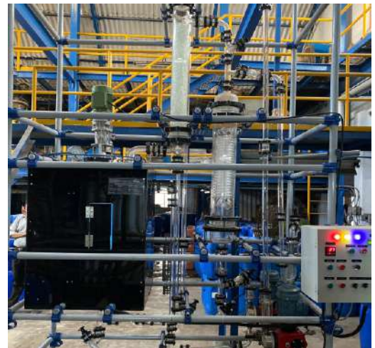
Continuous Photo-Chlorination Unit
