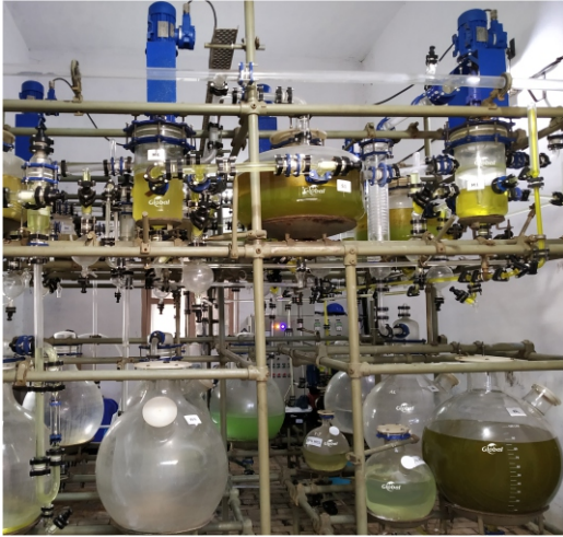
Phosphoric Acid Extraction Pilot Plant
