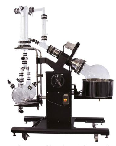
The rotation of the sphere which is flanged to the geared motor ensures an effective mixing of the product inside the vessel and wets the complete inner surface of the sphere, increasing the evaporation surface, therefore increasing the evaporation rate and hence shortening the evaporation time.
