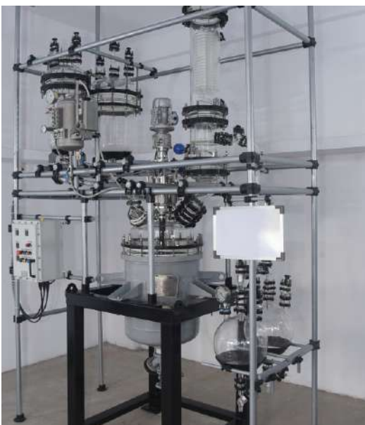
GLR Overhead Borosilicate Glass 3.3 Assembly
