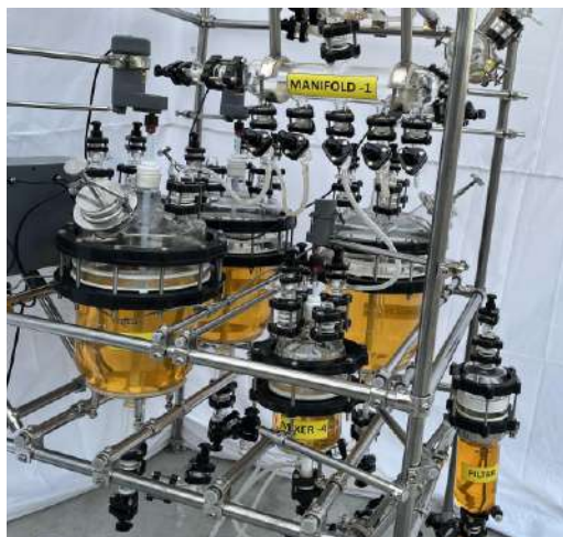
Custom Borosilicate glass 3.3 plant
